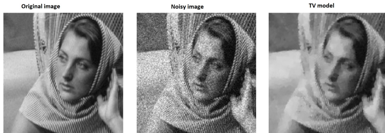
Figure : Staircassing artifacts produced by the TV regularization term
